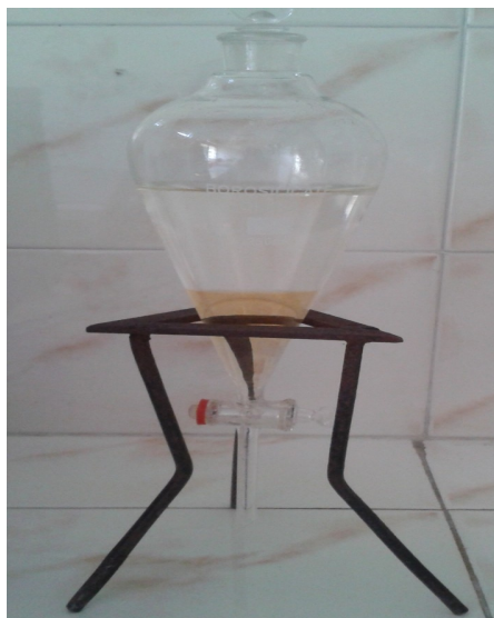
Fig. 1 Extraction of prodigiosin through separatory funnel
