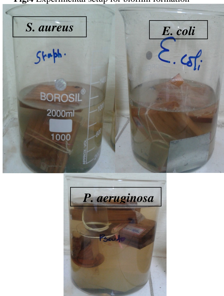
Fig.4 Experimental setup for biofilm formation
